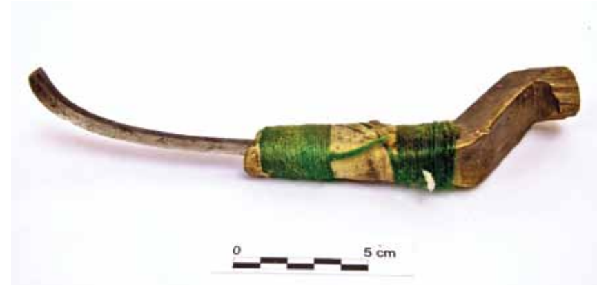
HANDLE OF A FILE TRANSFORMED INTO A CLAW TO REMOVE NAILS FROM A DWELLING FRAME
